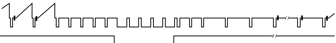
(b) 4th field CVBS output signal
